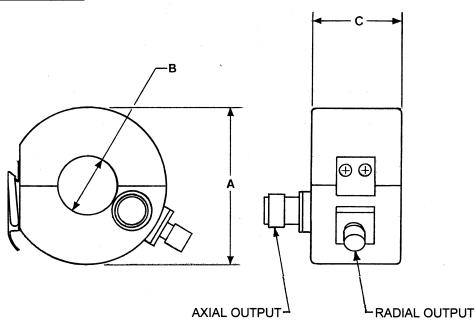
CONNECTOR OPTIONS: SMA, TNC, BNC (FEMALE) SPECIFY AXIAL OR RADIAL OUTPUT
