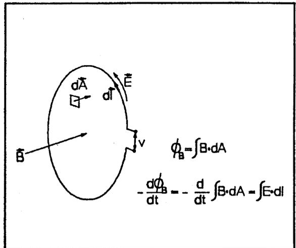
Figure 2. Conductive loop
